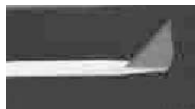
Unique "V" on the end of the tip allows accurate positioning of the tip. 60µm lever (foreground), 100µm lever (background).
