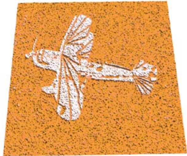
Figure 5: Pitts Model 12 biplane lithography on a sol-gel PZT thin film. Piezoresponse force microscopy (PFM) amplitude is painted on top of the rendered topography. 14.5µm scan, bitmapped lithography.
