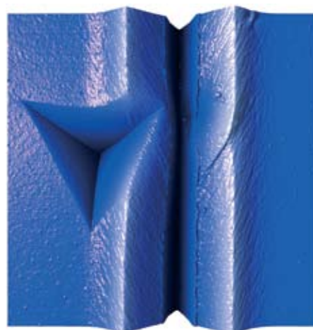
Figure 7: Indent and scratch on polyurethane, 17µm scan.
