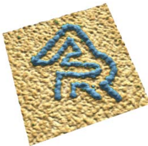
Figure 6: Anodic oxidation lithography on silicon, written in AC mode, 1µm scan.
