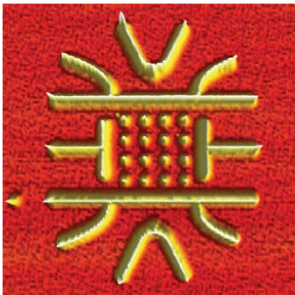
Quantum dot structure created on a GaAs wafer using oxidation lithography, 2.5 \mu m scan. Image courtesy D. Graf and R. Shleser, Ensslin Group, ETH Zurich.
