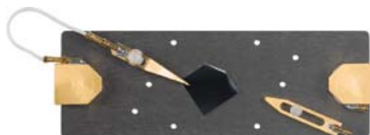
ORCA Sample Mount (top), and Cantilever Holder (left).
