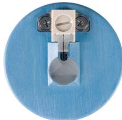
Ztherm dual-contact, differential drive cantilever holder. Compatible with and allows easy exchange of Anasys ThermaLever probes.
